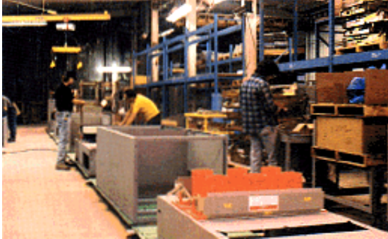
Metal-Clad Switchgear Assembly Line
